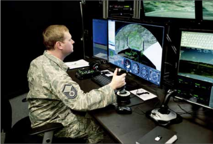
Master Sgt. Christopher Johnson flies a simulator during a training scenario, utilizing the AAJTS. The AAJTS system encompasses high fidelity visual displays, geo-specific visual data bases, equipment emulators, and associated hardware and software.
